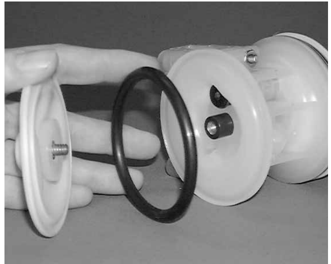
PTFE diaphragm configuration Figure 2
