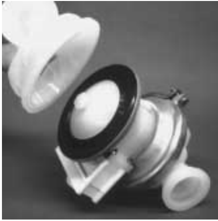
Step 10. Figure 10 Lift liquid chamber away from center section to expose diaphragm and outer piston. ( Figure 10 )
