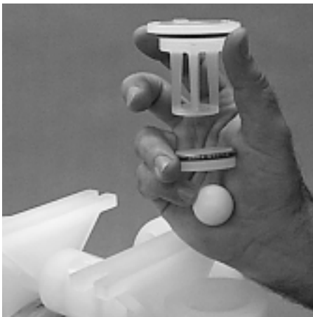
Step 6. Figure 6 Remove the bottom liquid retainer and retainer O-rings, discharge valve balls, seats and valve seat O-rings from the liquid chamber and inspect for nicks, gouges, chemical attack or abrasive wear. Replace worn parts with genuine Wilden parts for reliable performance. ( Figure 6 )
