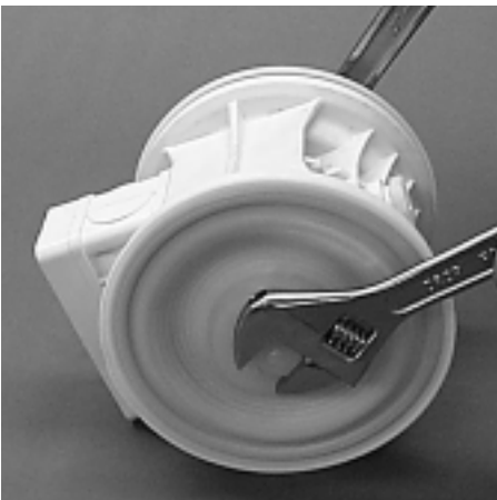
Step 11. Figure 11 Using two 1" sockets, remove diaphragm assembly from center section assembly. (Figure 11)
