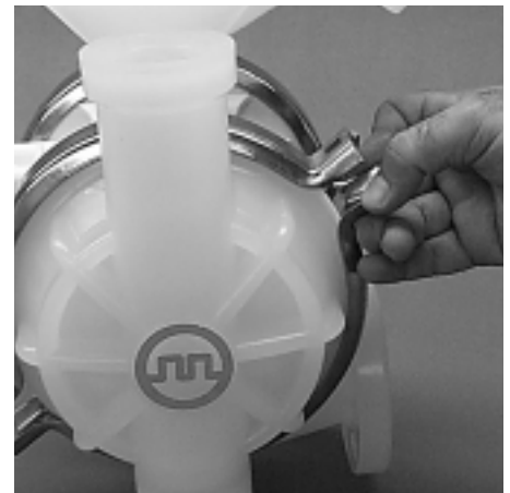
Step 8. Figure 8 Rotate the clamp bands so that they can be removed. ( Figure 8 )
