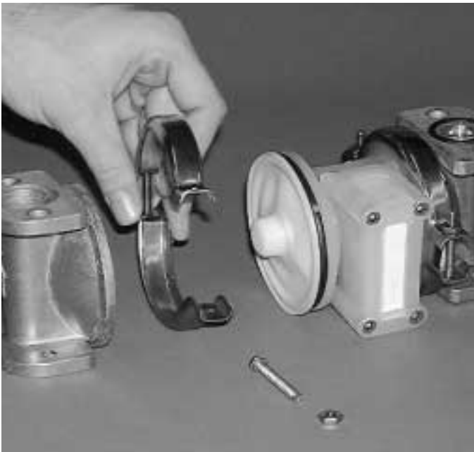
Step 7. Figure 7 After clamp bands are removed, pull chambers away from center section ( Figure 7 ).
