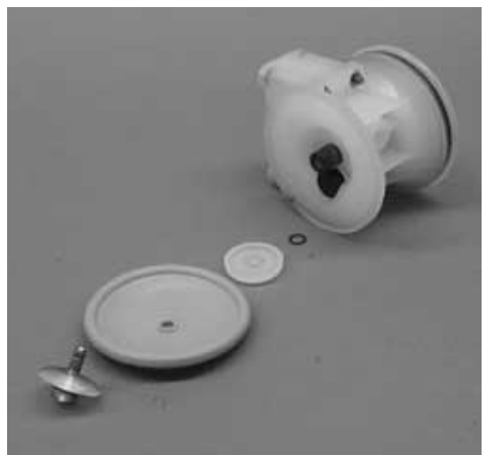
Step 10. Figure 10 For Rubber / TPE fitted pumps, remove the outer piston with \frac{7}{16} " wrench. You are now able to remove the complete assembly. Inspection of diaphragms and outer pistons is now possible.
