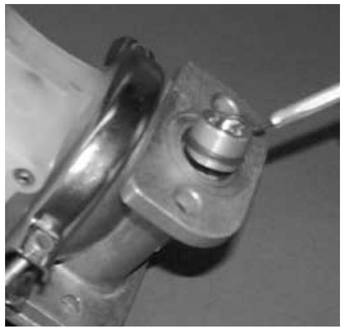
Step 4a. Figure 4a To remove top and bottom valve seats, on stainless steel or Hastelloy® pumps, use an O-ring pick and pull seats out from top to bottom or use 3/16" rod and push seats through. ( Figure 4a )
